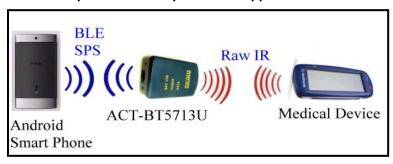
ACT-BT5713U-v2 enables any devices with BLE capability to connect with Raw IR devices.
